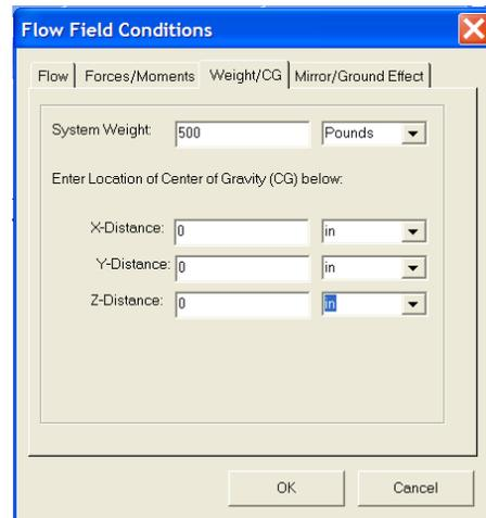
Figure 14: The CG Locations is used as a reference point.
