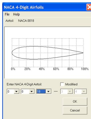
Figure 10: NACA 4-Digit Airfoils Dialog Box
