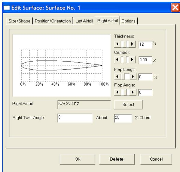
Figure 8: Right Airfoil Tab
