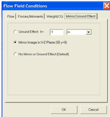
Figure 15: Modeling the hull with the mirror image setting.
