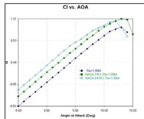
Figure 2. Lift Coefficient Versus Angle of Attack
