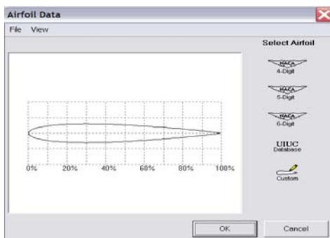
The dialog box can be used to select NACA 4, 5 & 6-Digit airfoils in addition to airfoils from the UIUC airfoil database and custom shapes.
